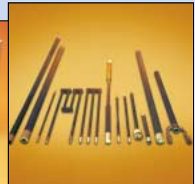
Silicon Carbide Hot Rod, Crusilite, Globar, Silit and multileg silicon carbide heating elements for furnace temp between 700 and 1650 °C, 1290 and 3000 °F.
