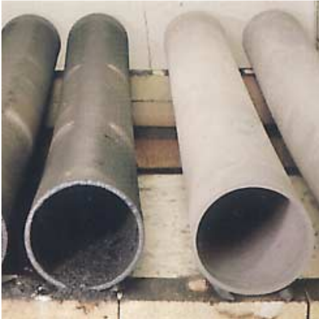
Comparison between NiCr tubes (left) and Kanthal APM tubes after 1000 hours at 1150 °C (2100 °F). The NiCr tubes are severely contaminated with oxide flakes as result of scaling while the APM tubes are still clean.
