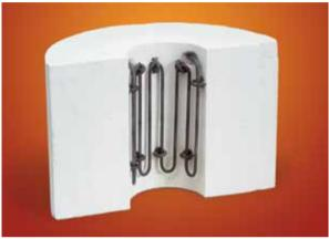
By using a newly developed special Kanthal<sup>®</sup> Super molybdenum disilicide (MoSi<sub>2</sub>) heating element material, the maximum temperature is now increased to 1725°C (3140°F) for Superthal HT half-cylinder type, enabling up to 1675°C (3050°F) furnace temperature.
