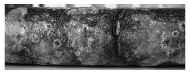
Conventional SiC element with eroded element surface.
