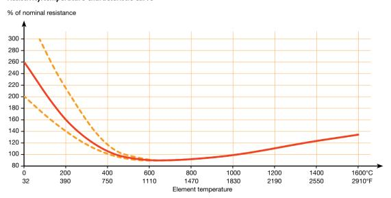
Fig. 9 Typical R/T curve.
