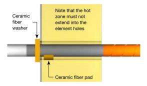
Fig. 5 Kanthal Globar SG element installed horizontal without sleeves.
