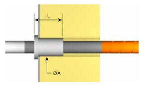
Fig. 4 Kanthal Globar SG element installed horizontal in sleeve.
