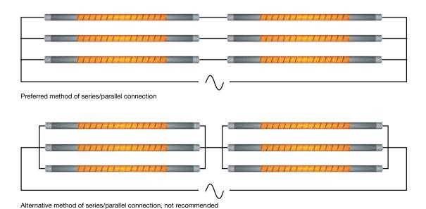
Fig. 11 Series/parallel connection.
