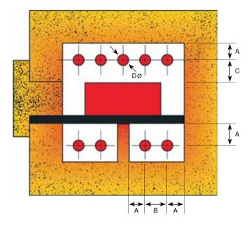
$A = (1.5 \times D) = Minimum$  spacing between element center and any adjacent refractory
