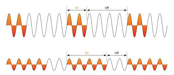
Fig. 18 Fast-cycle firing.
