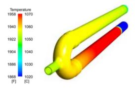
Temperature distribution in a conventional U-tube design.
