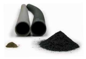
Visual differences in oxide spallation and sagging properties between the tube Kanthal APMT (left) and a standard FeNiCr tube after 2300 h at 1100°C (2010°F).
