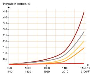
Carburized for 260 h in granular carbon
